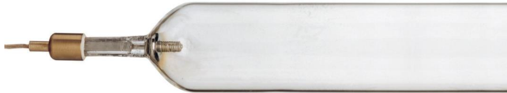
TQ Lamp: power range 4-60kW, metal base with lead, roll-seal
